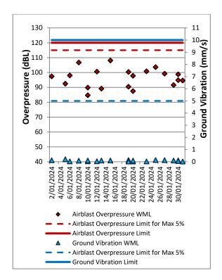
Figure 11: MTIE Blast Monitoring Results - January 2024
