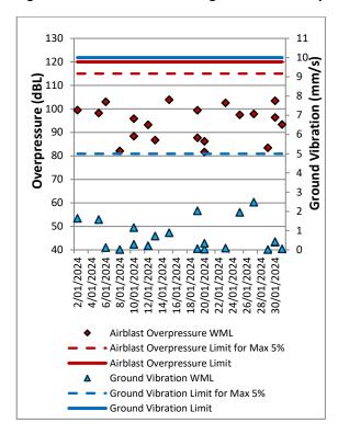
Figure 12: Wollemi Peak Road Blast Monitoring Results – January 2024
