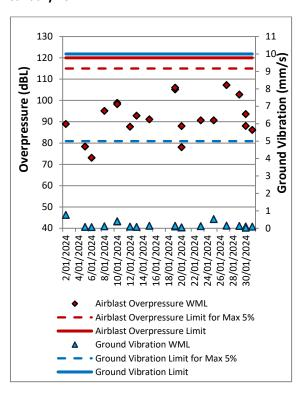
Figure 14: Warkworth Blast Monitoring Results – January 2024
