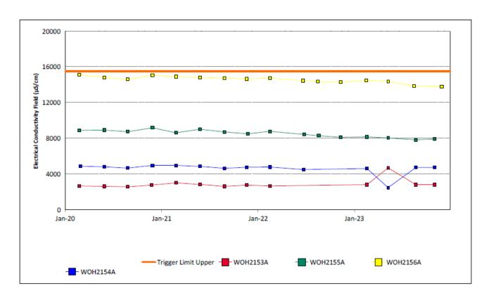
Figure 25: Redbank Seam Electrical Conductivity Field Trend – December 2023
