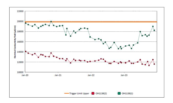
Figure 37: Warkworth Seam Electrical Conductivity Field Trend – December 2023
