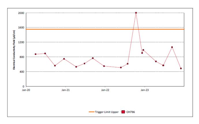
Figure 51: Hunter River Alluvium 1 Electrical Conductivity Field Trend – December 2023
