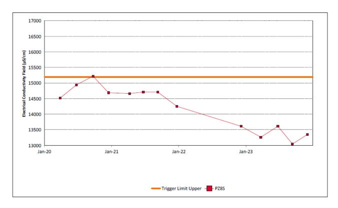
Figure 40: Wollombi Alluvium 1 Electrical Conductivity Field Trend – December 2023
