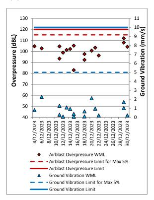
Figure 69: Wambo Road Blast Monitoring Results - December 2023
