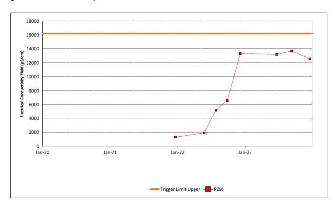
Figure 42: Wollombi Alluvium 2 Electrical Conductivity Field Trend – December 2023
