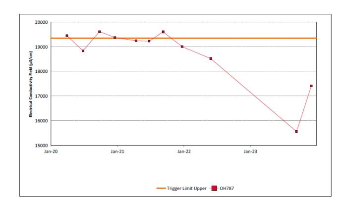
Figure 53: Hunter River Alluvium 2 Electrical Conductivity Field Trend - December 2023
