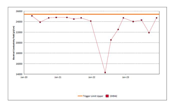
Figure 55: Hunter River Alluvium 3 Electrical Conductivity Field Trend – December 2023
