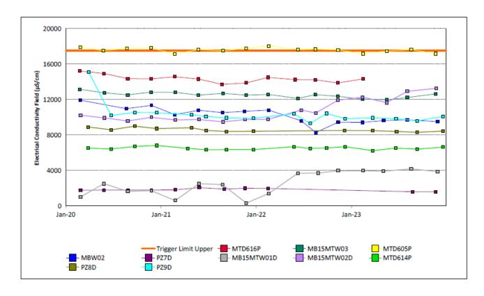
Figure 28: Shallow Overburden Electrical Conductivity Field Trend – December 2023
