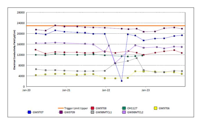
Figure 16: Bayswater Seam Electrical Conductivity Field Trend – December 2023
